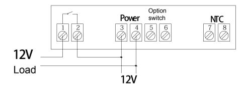
Terminals 1 and 2: Normally opened contact of relay
